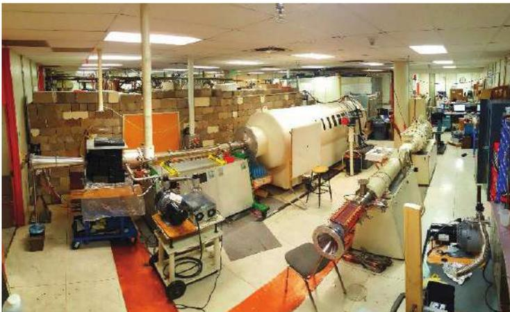
UNM has two accelerators in its Pulsed Power, Beams, and Microwaves Laboratory: a modified PI-110A Marx generator with pulse forming line, and a SINUS-6 Tesla-transformer with a pulse forming line, a low impedance version to study relativistic magnetrons and a high impedance one to study Cherenkov devices. The photograph below shows both of these accelerators. UNM also has a complete array of advanced instrumentation for pulsed power, plasma, and electromagnetic diagnostics.
